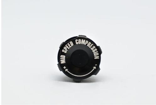
**Caution: the adjustment is always made from the closed/screwed down position and we count down the number of revolutions.**
