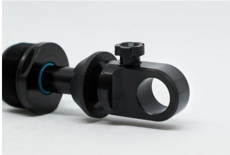
**Caution: the adjustment is always made from the closed/screwed down position and the number of clicks is counted down.**
